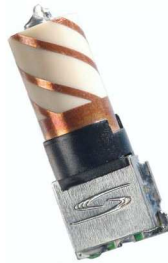
Figure 2 – Sarantel helix antenna (cover removed)
